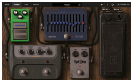
The B-3X includes five handy stomp-box effects that can be placed between the organ and the cabinet
