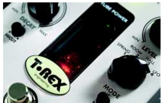
The Room-Mate's green on/off LED will turn red if the input signal is too high
