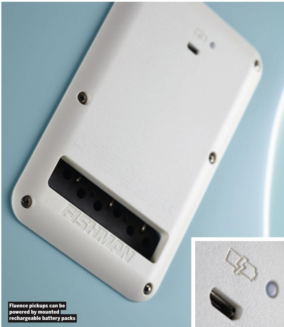
Fluence pickups can be powered by mounted rechargeable battery packs
