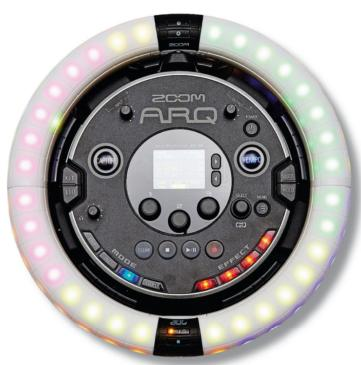
TRIGGERS The Effects triggers on the Ring Controller combine with its Accelerometer to let you manipulate effects on the fly
