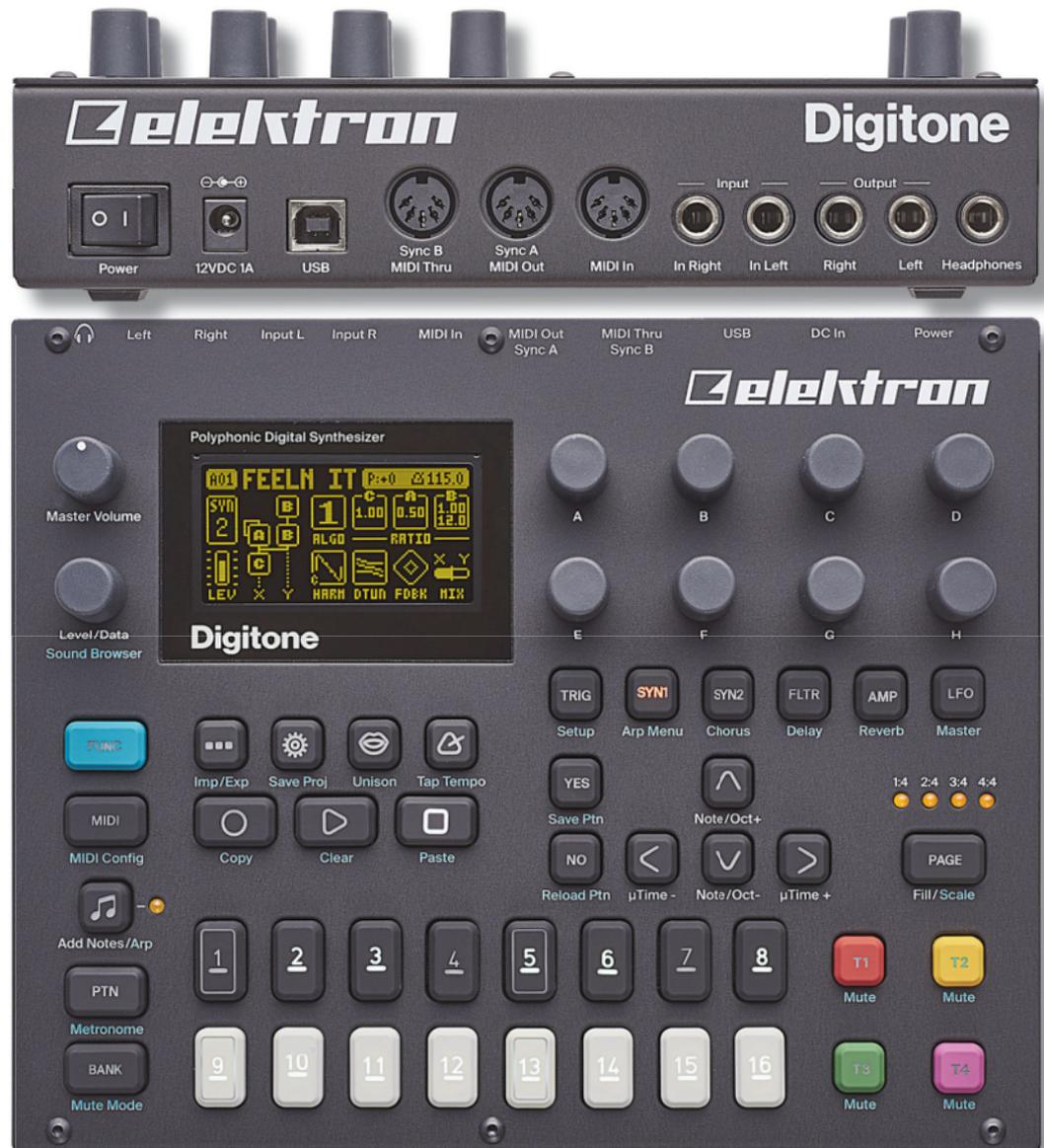
**FM ENGINE:** A four-operator, eight-algorithm affair with plenty of tweakable parameters
