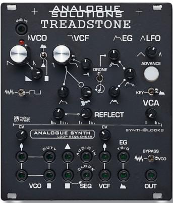
does pack a lot of features. The real boon is the 16-note step sequencer. You can use MIDI clock or incoming analogue clock for the tempo and notes are simply entered using MIDI note-on messages. Other triggering options on the Treadstone are the LFO and drone functions.
