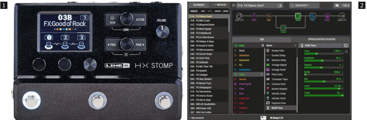
3. The three soft knobs are assigned to functions and values in the screen above, and have both push and turn actions
