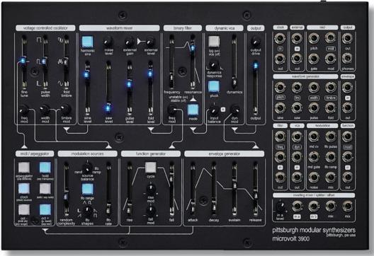
ARP: You wouldn't know it from looking at the four buttons, but there's a deceptively capable sequencer and arp onboard FILTER: The binary filter has built-in drive and an extended resonance range for plenty of grit
