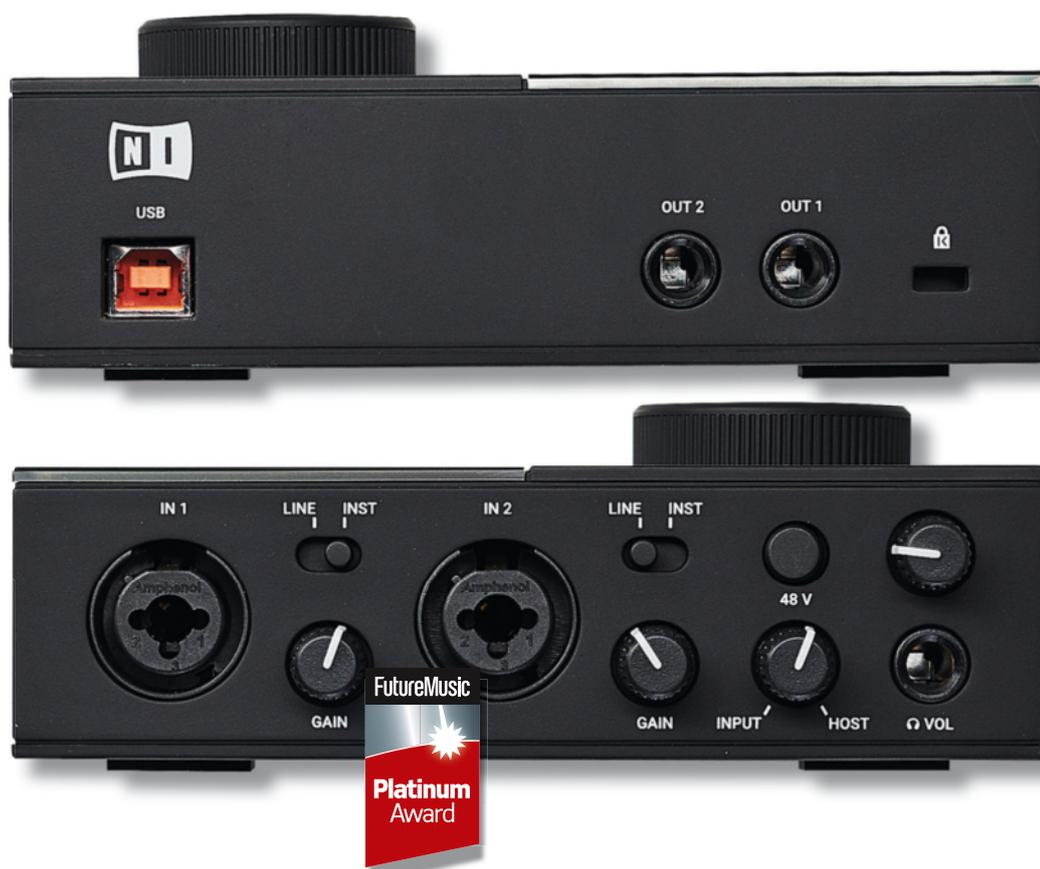
**K**omplete Audio 2 is one of a pair of new compact USB 2.0 bus-powered audio interfaces from Native Instruments. Both follow a similar desktop style design to their long established Komplete Audio 6 unit. However, the new interfaces are smaller, lighter and visually slicker, and although there's no onboard MIDI like the Audio 6, the maximum sampling rate has been increased to 192kHz.
