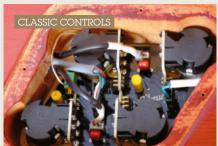
Connections from the pickups, three-way toggle switch and to the jack output are all push-fit. The large yellow caps 0.01 microfarad (103k) create the 'tap' function; the tone caps are smaller brown 0.022 microfarad (223k).
