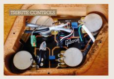
both-pickups-on position. However, with the neck pickup alone selected and the tap function engaged, if the neck tone control switch is down then the neck's inner slug coil is primarily voiced; pulling up the neck's tone control chooses the outer screw coil – a very subtle difference. The bridge pickup's tone control switch is a 'pure bypass' that connects the bridge pickup directly to the output jack.
