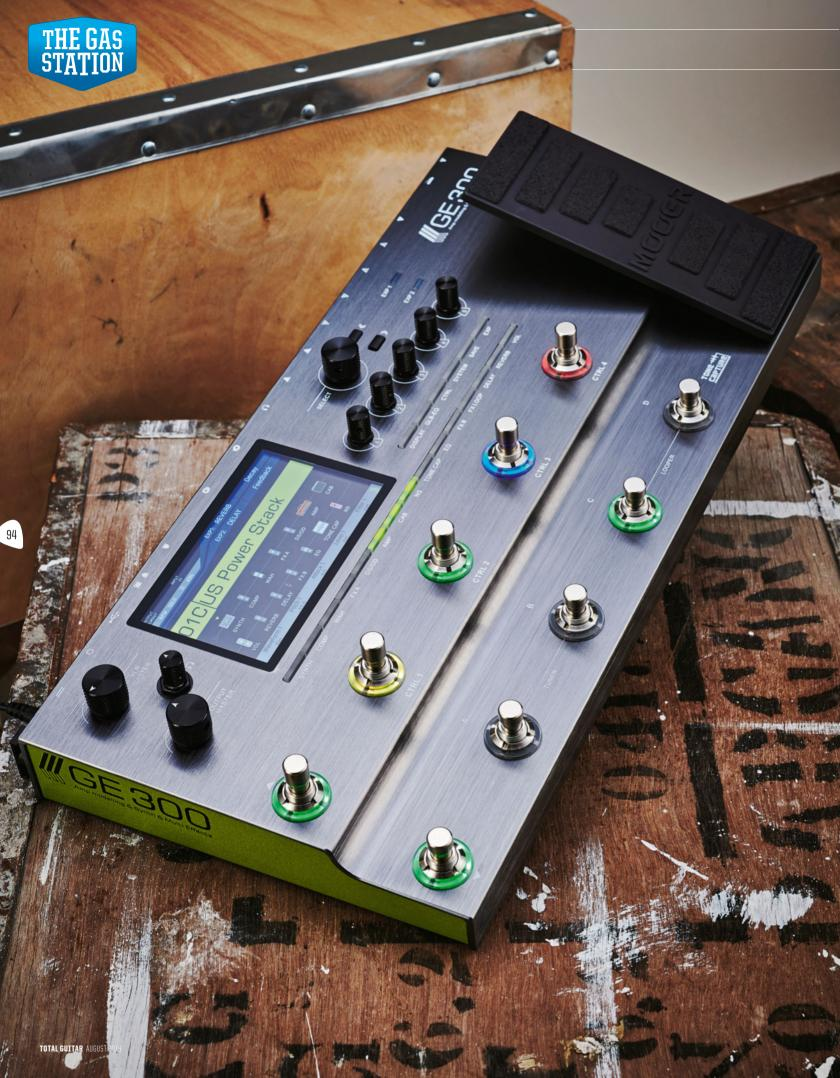
There's an integrated expression pedal, and, like on many other floorboards, on the rear there's an expansion port allowing for a second to be connected
