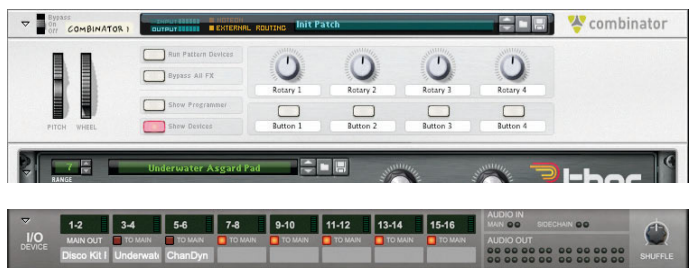
I/O BAR: The Reason Rack Plugin can have up to 16 stereo outputs, a stereo input and stereo sidechain input
