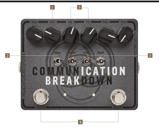
These knobs vary the voltage to the collector of the second transistor adjusting the fuzz from full and fat to a thinner gated tone
