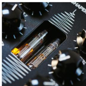
Valves introduce subtle variation into a circuit, where fluctuations can add some 'life' that digital components typically don't. An integral part of the Fusion sound is that they can be overdriven easily, for characteristic Erica punch and growl.
