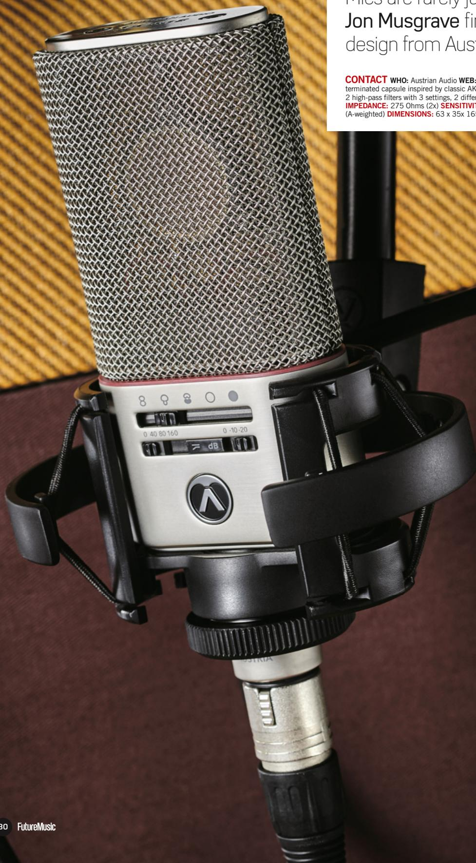
**O**C818 is a multipattern phantom-powered large-capsule condenser mic from Austrian Audio. It uses their own handbuilt CKR12 dual diaphragm ceramic capsule, heavily influenced by the classic AKG CK12. The mic has four pattern options (figure 8, supercardioid, cardioid and omnidirectional) with on-body high-pass filter and level pad. The Studio Set kit on review included a foam windshield, shockmount, regular mic clip, mini XLR cable and lightweight flight case.
