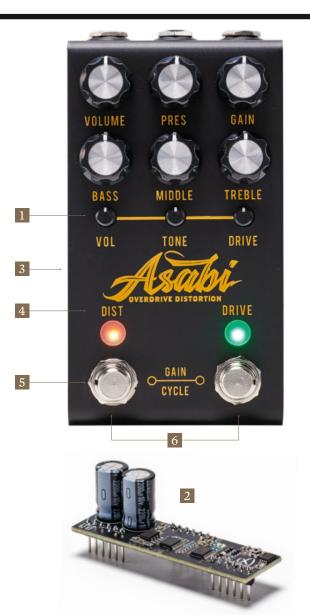
Tech Spec **ORIGIN: USA** TYPE: Overdrive/ distortion pedal FEATURES: True bypass, plug-in alternative circuit boards **CONTROLS:** Volume, Presence, Gain, Bass, Middle, Treble, Overdrive Volume, Overdrive Tone, Overdrive Drive, Distortion footswitch, Drive footswitch **CONNECTIONS:** Standard input, standard output, MIDI POWER: 9V DC adaptor - pedal requires 120mA minimum DIMENSIONS: 67 (w) x 124 (d) x 70mm (h)
